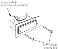
**4** Lower the removal tool toward the bottom, and pull out the unit halfway while pressing towards the inside.
